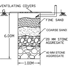
RAIN WATER HARVESTING STUCTURE DETAILS
